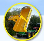
2 door opening options to meet all your needs: manual opening of the 2 door parts or hydraulic opening of the high-clearance door
